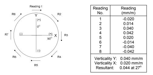
It can be demonstrated that the following formulas apply for the case with 8 tangential readings.
